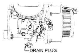
Figure 9. Drain Plug
